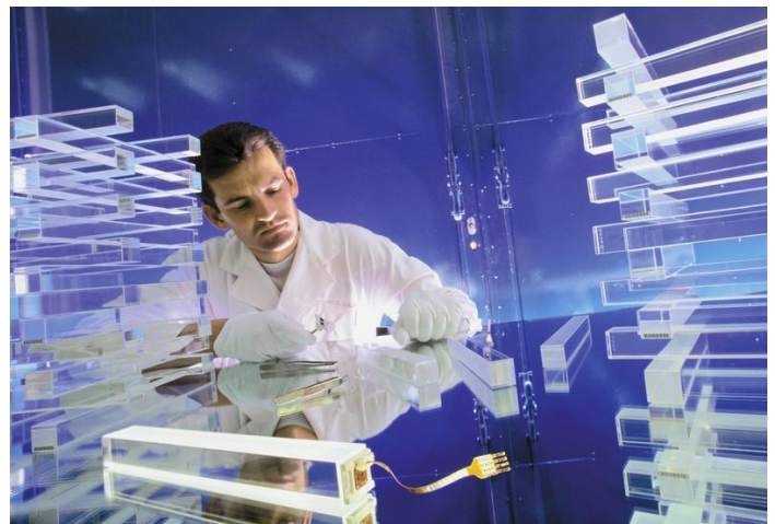
Figure 1 – Scintillating crystals for particle detectors (in this example, for CMS experiment at LHC) are also used in PET scanners. Photo by Peter Ginter (2004). Credit: CERN ( cds.cern.ch/record/808282 ).
