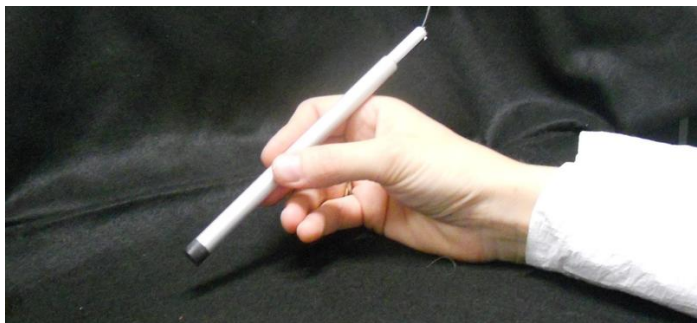
Figure 2 – Prototype of the probe that, enveloped in a sterile covering, should be used by the surgeon during the procedure to verify the completeness of the tumor resection.
